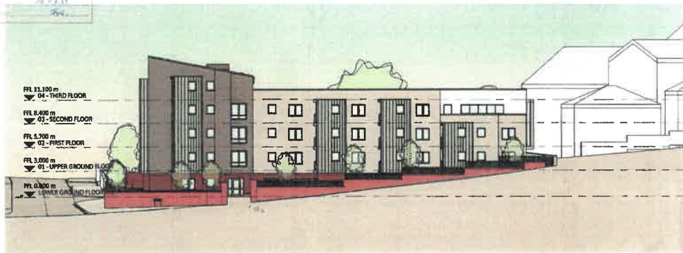
1 | NORTH-EAST ELEVATION - FACING FFORDD FARRAR SCALE: 1:200
